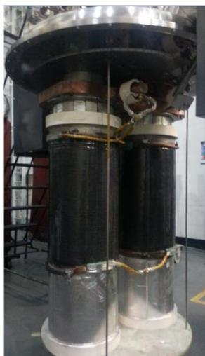
Figure 8: 11 kV SFCL coil using  $MgB_2$  superconductor at University of Manchester
