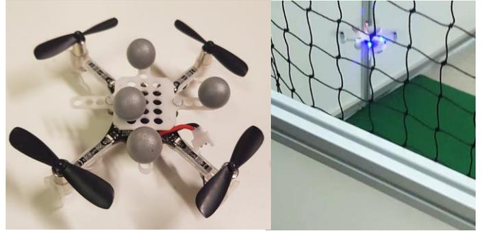
Figure 2: A Crazyflie Drone equipped with VICON markers.
