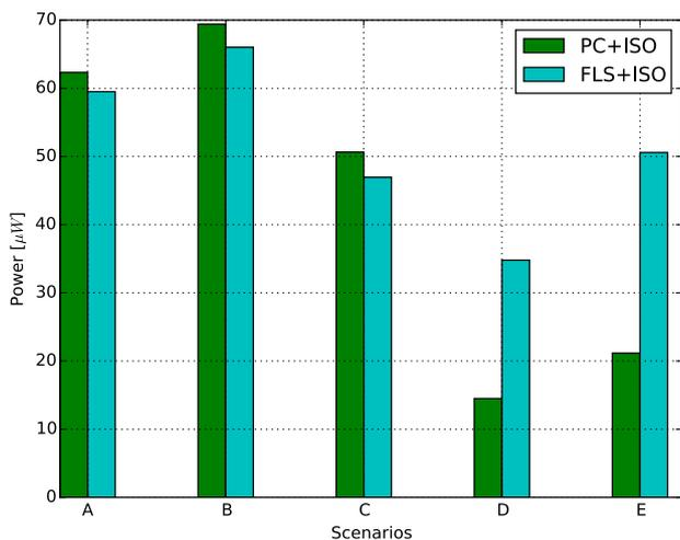
Fig. 5. Power dissipation of the proposed circuit compared to traditional level conversion circuits where isolation cells are also connected in series with the shifters.
