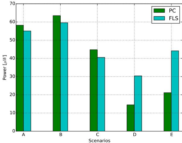
Fig. 4. Power dissipation of the proposed by-pass circuit compared to traditional level-up shifters.
