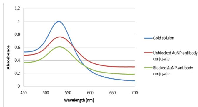
Fig. 2. The Visible-spectrum of AuNP, unblocked AuNP-antibody conjugates and blocked AuNP-antibody conjugates
