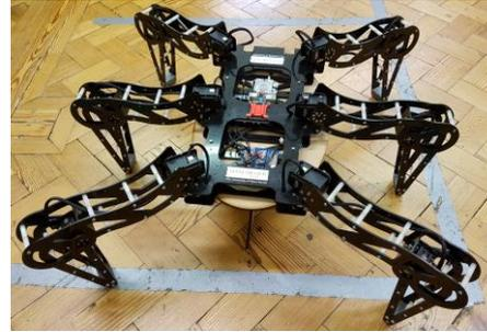
Fig. 1. CORIN mobile robot.
