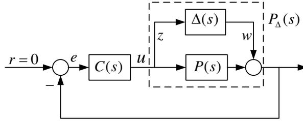
Figure 3.3: Controlled closed-loop system
