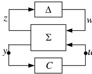
Figure 3.4: Rearranged LFT interconnection
