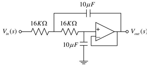
Figure 1.1: A Sallen-Key low-pass filter
