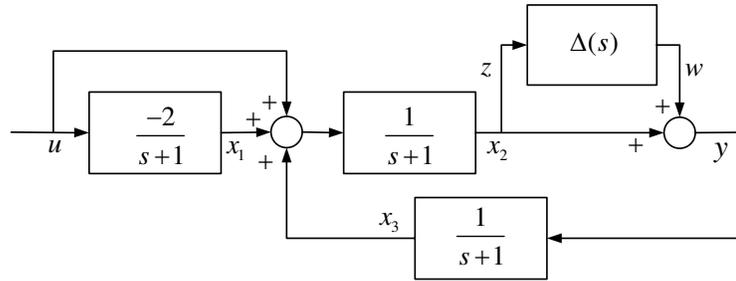
Figure 5.3: Block diagram of an uncertain system to be controlled by means of a state-feedback controller to be constructed using an LMI approach.
