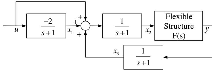
Figure 5.2: Block diagram of a system to be controlled using a state-feedback LMI approach to robust controller design.
