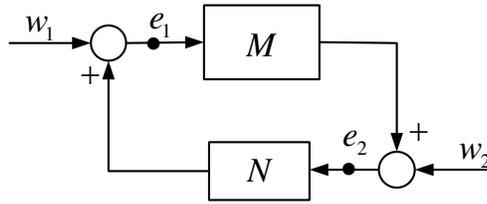
Figure 2.7: A positive feedback interconnection
