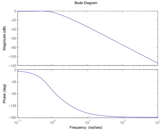
Figure 5.4: Bode plot of the closed-loop transfer function  $G_{cl}(s)$  from the  $w$  to  $z$ .
