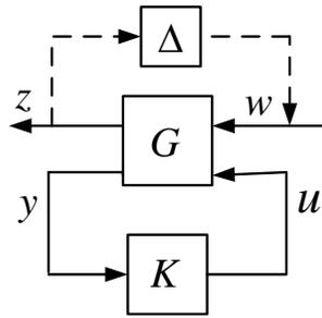
Figure 2.4: An LFT interconnection for robust control
