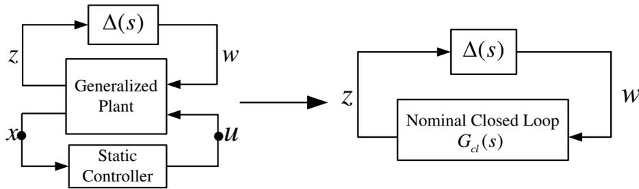
Figure 5.1: A feedback control system where the plant uncertainty  $\Delta(s)$  is strictly negative-imaginary, and satisfies  $\Delta(\infty) \geq 0$ .
