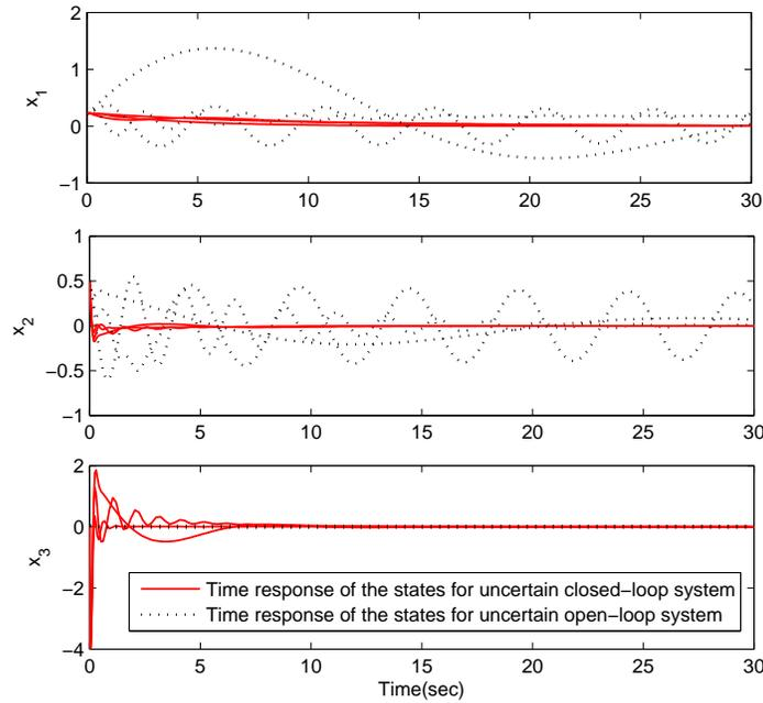
Figure 5.10: Open-loop responses and closed-loop responses of the uncertain system with three randomly chosen parameter of  $J_2$ ,  $k_2$  and  $d_2$  under a nonzero initial condition.
