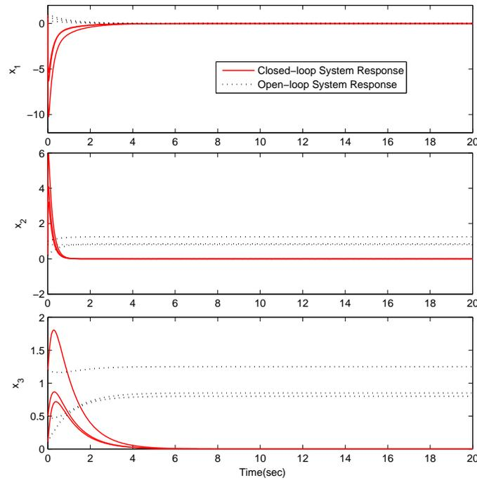
Figure 5.5: Open-loop responses and closed-loop responses of the nominal system under three randomly chosen nonzero initial states.
