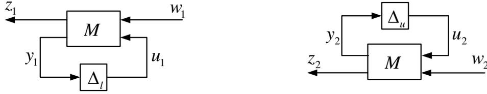
Figure 2.1: LFT diagram representations of lower and upper LFT
