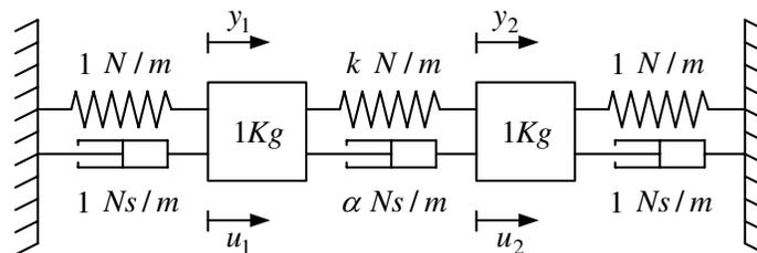
Figure 3.2: Lightly damped uncertain mechanical plant
