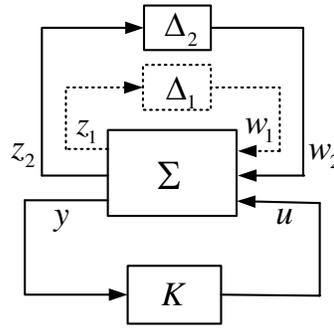
Figure 4.1: An LFT interconnection for performance analysis
