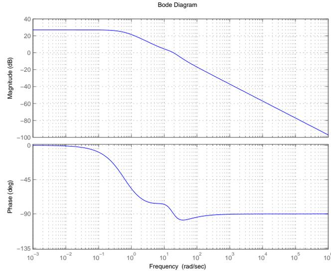
Figure 5.9: Bode plot of the closed-loop transfer function  $G_{cl}(s)$  from the uncertainty output  $w$  to the uncertainty input  $z'$ .
