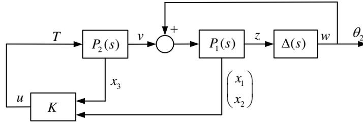
Figure 5.7: Block diagram of an uncertain two-mass model controlled via state-feedback.
