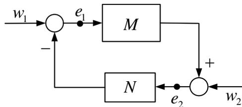
Figure 2.6: Feedback interconnection of passive systems
