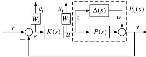
Figure 4.4: Controlled closed-loop system
