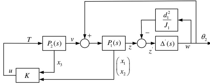
Figure 5.8: Block diagram of an uncertain tow-mass system by means of state-feedback control.
