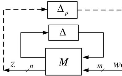
Figure 2.5: An LFT interconnection for  $\mu$  robust performance analysis
