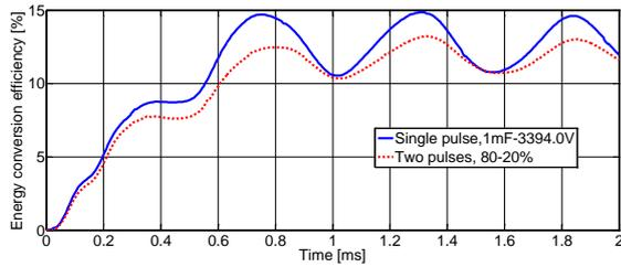
Fig. 12: Single pulse, double pulse energy conversion efficiency comparison.
