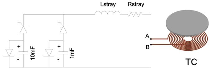
Fig. 9: Two discharge stages circuit, schematic representation.
