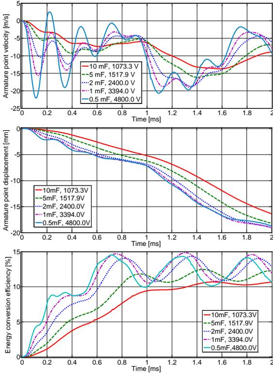
Fig. 6: TC actuator velocity (top), displacement (middle) and energy conversion efficiency (bottom).
