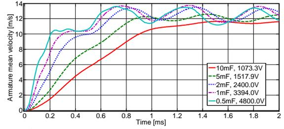
Fig. 8: TC armature's mean velocity.
