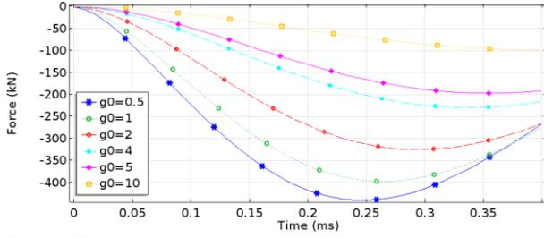
Fig. 5: TC armature electromagnetic force for different coil-armature gaps.
