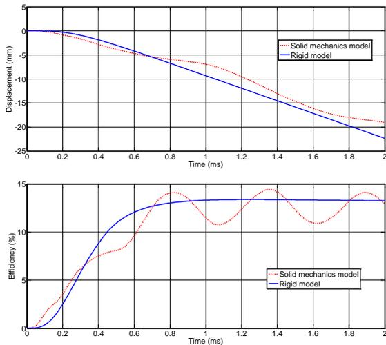
Fig. 4: Electrical to mechanical energy conversion efficiency (top) and armature displacement (bottom) comparison for the TC with and without considering material bending.
