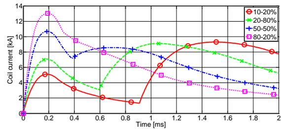
Fig. 10: Coil current traces from the double pulse setup cases.
