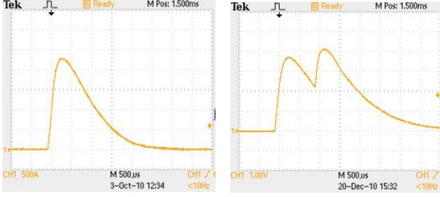
Fig. 2: Example coil excitation current, single discharge (left) and two stage discharge (right) [7].
