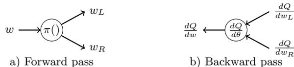
Fig. 1: During the forward pass (root to leaves), weights are calculated. During the backward pass (leaves to root), gradients are calculated.
