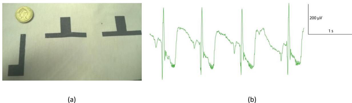
**Figure 1 Graphene printed electrodes on textile substrates for bio-sensing without requiring a fixed connection to the body**
