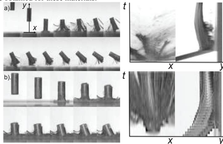
**FIGURE 1.** Impact onto 0° composite Taylor cylinders. a). impacts 148 & b). 268 m s<sup>-1</sup>. IFT 33 μs. Streak (*x-t*) images to right.
