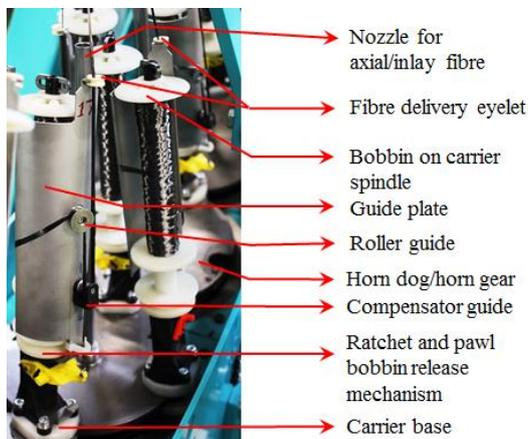
Fig. 3: Different components of a radial braider carrier
