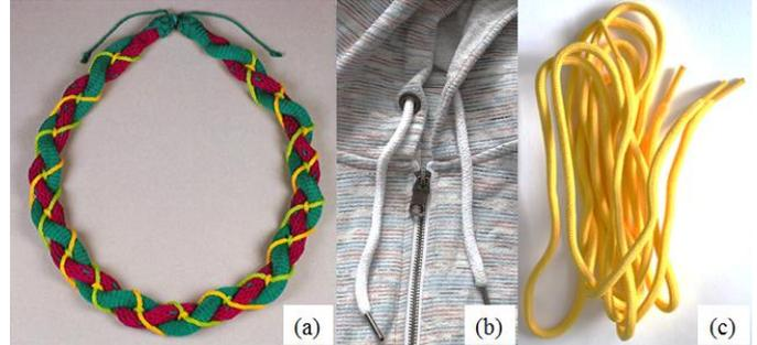
Fig.6 Examples of braided textile (a) Fancy (Versatile) braid[15] (b) drawstring for jacket (c) shoelace
