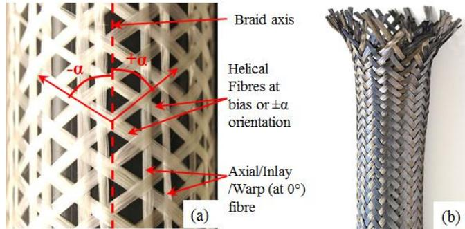
Fig. 5: (a) Glass fibres at different orientation in a braid with braid angle ( $\pm\alpha$ ) and braid axis which is same as the machine as well as longitudinal axis of the core (b) Carbon fibre braided sleeve
