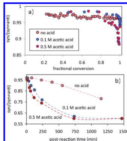
**Figure 4.** Syn/anti selectivity in the Michael reaction in Scheme 1 under the conditions given in Figure 2 and acetic acid concentrations as shown, as a function of (a) fraction conversion *during* reaction and (b) time *after* reaction completion.
