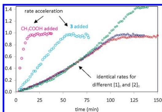
**Figure 2.** Temporal concentration of product 3 in the reaction in Scheme 1 monitored by  $^1\text{H}$  NMR spectroscopy. Red circles:  $[1]_0 = 1.2$  M,  $[2]_0 = 1.0$  M. Blue circles:  $[1]_0 = 1.7$  M,  $[2]_0 = 1.0$  M. Green circles:  $[1]_0 = 1.7$  M,  $[2]_0 = 1.5$  M. Turquoise circles: same as red circles, with 0.5 M 3 added. Pink circles: same as red circles, with 0.1 M  $\text{CH}_3\text{COOH}$  added. Catalyst loading is  $[4] = 0.1$  M in all cases.
