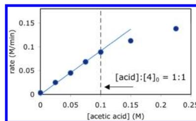
**Figure 3.** Effect of added acid concentration on reaction rate for the reaction in Scheme 1 with  $[1] = 1.2$  M,  $[2] = 1.0$  M, and  $[4] = 0.1$  M. Rate measured from reaction calorimetric profiles at 20% conversion.
