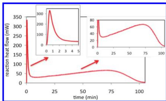
**Figure 1.** Temporal reaction rate in the reaction in Scheme 1 with initial concentrations  $[1]_0 = 1.7$  M,  $[2]_0 = 1.5$  M, and  $[4] = 0.1$  M monitored by reaction calorimetry, showing an initial spike in rate (left inset) and the subsequent accelerating rate profile (right inset).
