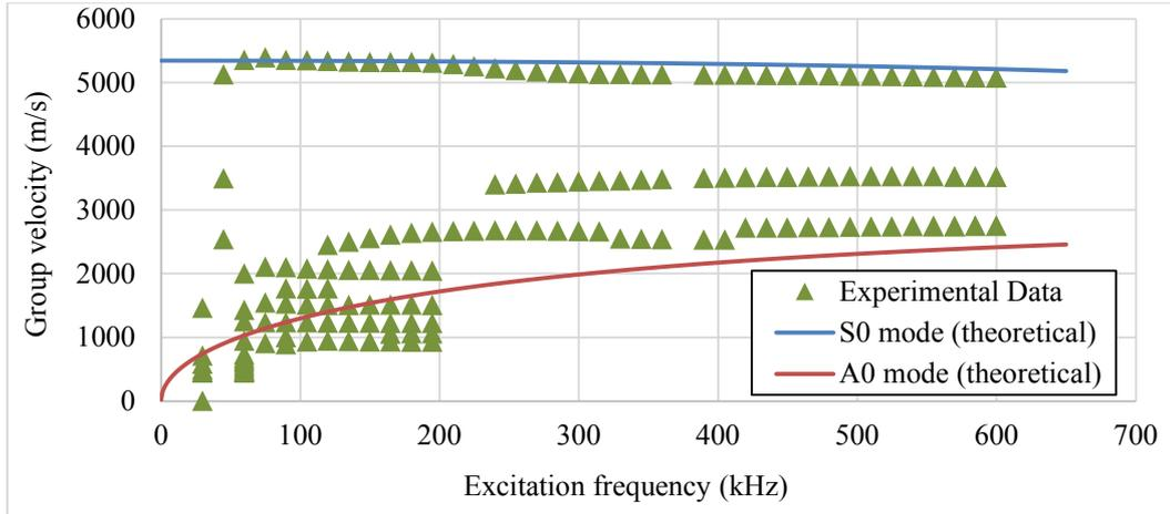
Figure 2: Dispersion curves of the aluminium plate.
