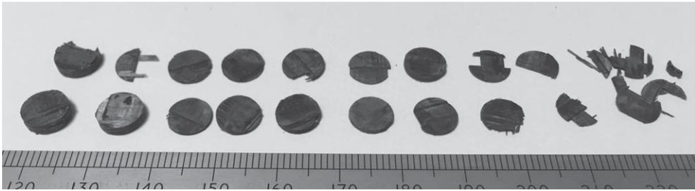
**Figure 7.** Recovered discs from the impact of a TT cylinder at a velocity of  $246 \text{ m s}^{-1}$  (see sequence figure 6b).
