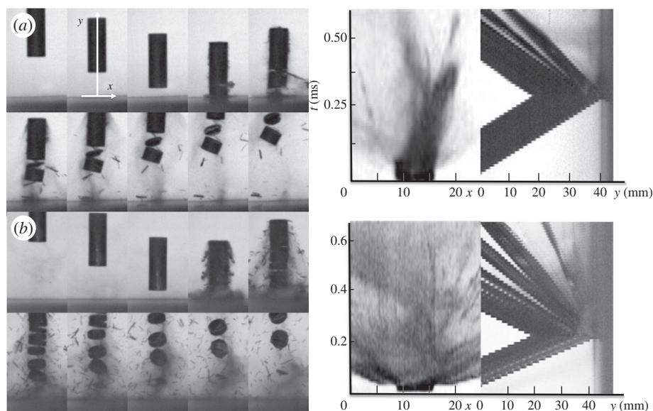
**Figure 6.** (left) Impacts onto through-thickness (TT) composite cylinders. (a) IFT  $42 \mu\text{s}$  impact velocity  $153 \text{ m s}^{-1}$  and (b) IFT  $42 \mu\text{s}$  impact velocity  $246 \text{ m s}^{-1}$  (right) streak images for the  $x$ - and  $y$ -axes.
