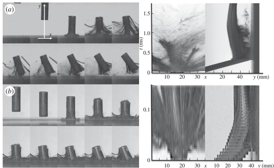
**Figure 4.** Impact response of  $0^\circ$  composite Taylor cylinders. Impact at (a)  $148 \text{ m s}^{-1}$  and IFT =  $125 \mu\text{s}$  and (b) at  $268 \text{ m s}^{-1}$  and IFT =  $17 \mu\text{s}$  (left) successive time frame images and (right) streak images for  $x$ - and  $y$ -directions shown to the right with common time axis,  $t$ , for each impact.
