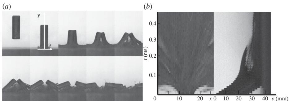
**Figure 5.** (a) Time-lapse sequence showing the impact response of a  $45^\circ$  composite cylinder. The IFT for this sequence is  $42 \mu\text{s}$  per frame and the impact velocity  $213 \text{ m s}^{-1}$ , (b) streaks for the  $x$ - and  $y$ -axes (cf. figure 4b).
