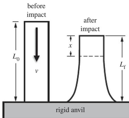
**Figure 1.** The Taylor impact test [6]. A right cylinder is projected onto a rigid anvil and inelastic deformation in the shocked zone at the impact face deforms it and instigates damage in various modes as waves equilibrate the stress state within the cylinder.
