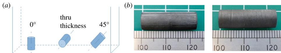
**Figure 2.** Carbon-fibre composite Taylor samples; (a) cylinder orientations with respect to the composite plate, (b) in-plane  $0^\circ$  and through-thickness (TT) samples before firing. (Online version in colour.)
