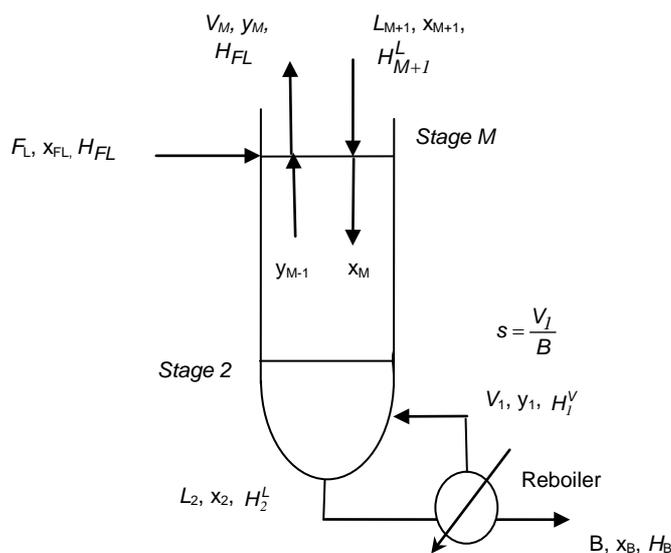
Figure 2. Schematic representation of the stripping section
