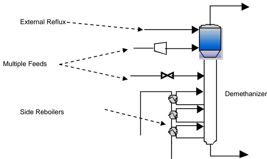
Figure 1. A typical demethanizer column
