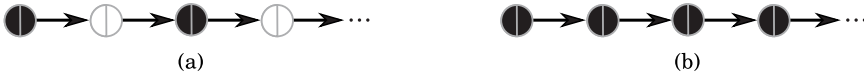
Fig. 2. Locality of write accesses in a chain of dependent tasks. (a) Tasks with buffers allocated on alternating nodes. (b) Task buffers allocated on the same node.
