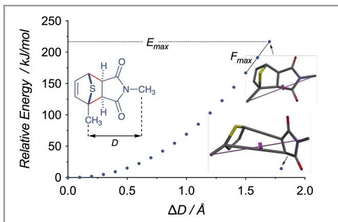
**Figure 2.** CoGEF calculation (DFT B3LYP/6-31G\*) for the *S*-prox-exo adduct. Scissile bonds shown in red.  $F_{\max}$  is calculated from the slope around  $E_{\max}$ . Structures at  $E_{\max}$  and after scission shown (hydrogen atoms omitted for clarity).
