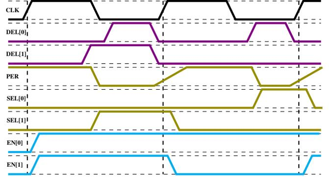
Fig. 4: Signal propagation of the encoder circuit.
