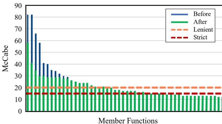
Figure 3: Plot of the 50 most complex class member functions in Merlin++ identified by Metriculator before and after complexity reduction refactoring.
