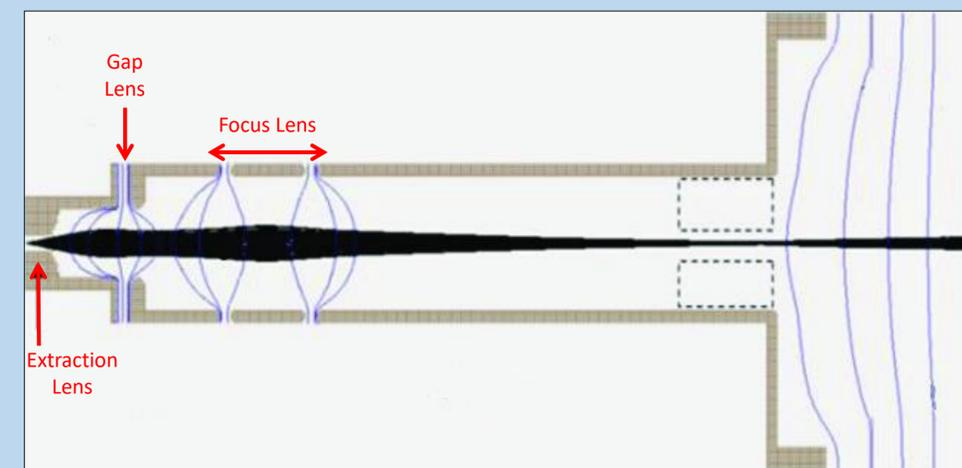
Once we have made an ion beam from the TORVIS, we use a series of electromagnetic lenses (Extraction, Gap, Focus) to position and focus the beam as desired, ready for accelerating. These lenses do much the same thing as optical lenses, though with electric and magnetic fields.
