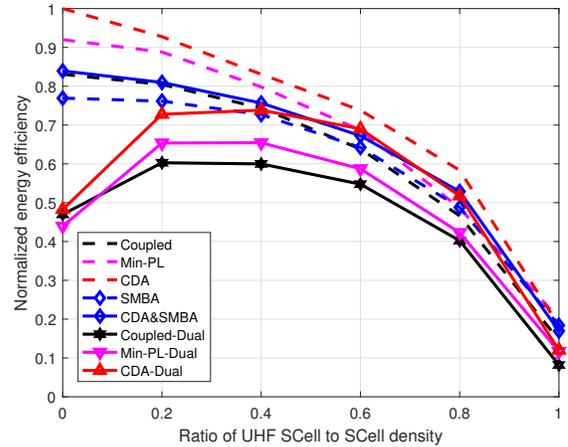
Fig. 8: Normalized network energy efficiency when the UHF SCells make up different proportions of all the SCells ( $\beta = 5$ ).
