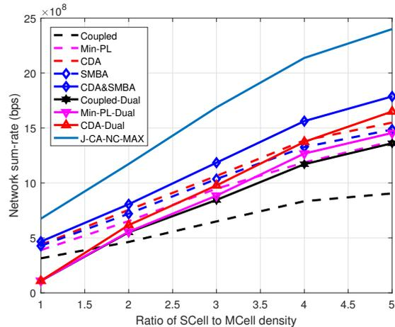
Fig. 6: Network sum-rate in the UL vs. ratio of SCell density to MCell density in single and dual connectivity scenarios ( $\gamma = 0.5$ ).
