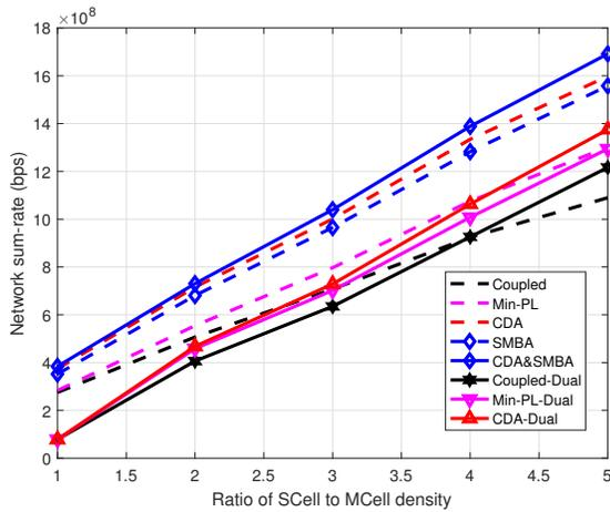
Fig. 13: Network sum-rate in the UL vs. ratio of SCell density to MCell density in single and dual connectivity scenarios (less density scenario,  $\gamma = 0.5$ ).
