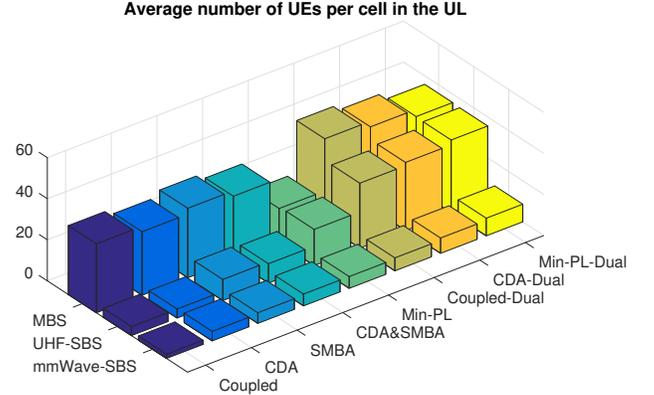
Fig. 2: Average number of UEs per cell in the UL for different association schemes in single and dual connectivity scenarios ( $\beta = 2$ ,  $\gamma = 0.5$ ).
