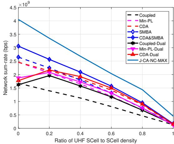
Fig. 7: Network sum-rate in the UL vs. ratio of UHF SCell density to SCell density in single and dual connectivity scenarios ( $\beta = 5$ ).
