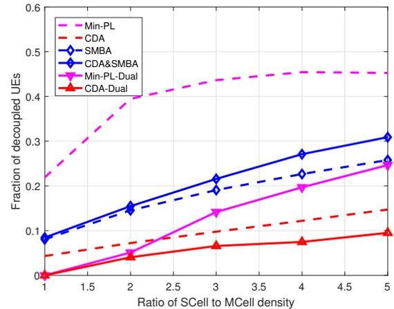
Fig. 4: Ratio of UEs decoupled in the UL and DL vs. ratio of SCell density to MCell density ( $\gamma = 0.5$ ).
