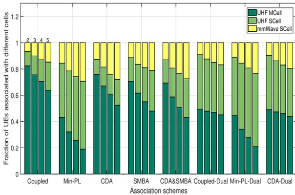
Fig. 3: Ratio of UEs associated with different BSs at different ratios of SCell density to MCell density and association schemes ( $\gamma = 0.5$ ).
