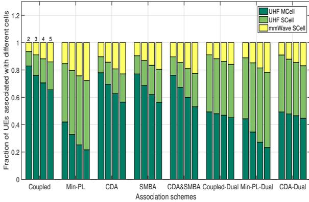
Fig. 12: Ratio of UEs associated with different BSs at different ratios of SCell density to MCell density and association schemes (less density scenario,  $\gamma = 0.5$ ).
