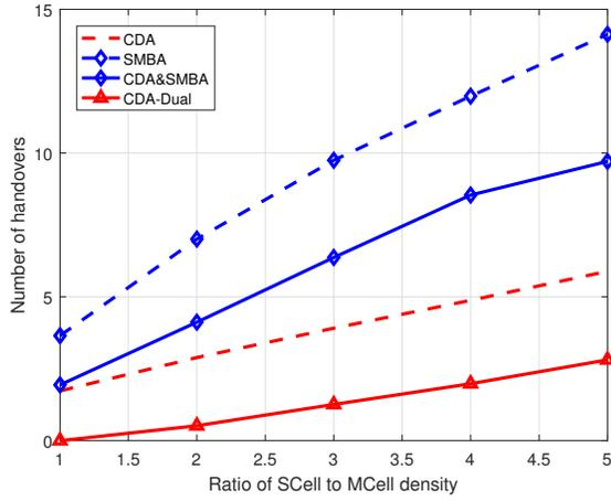
Fig. 9: Number of handovers in the UL vs. ratio of SCell density to MCell density in single and dual connectivity scenarios ( $\gamma = 0.5$ ).
